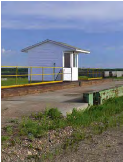
Truck scales at Large Feedlot with 150-ton capacity.
